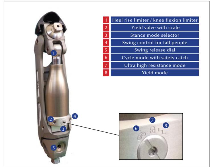
Fig 1: Adaptive  $\alpha$ -logic Control Hydraulic Knee.
